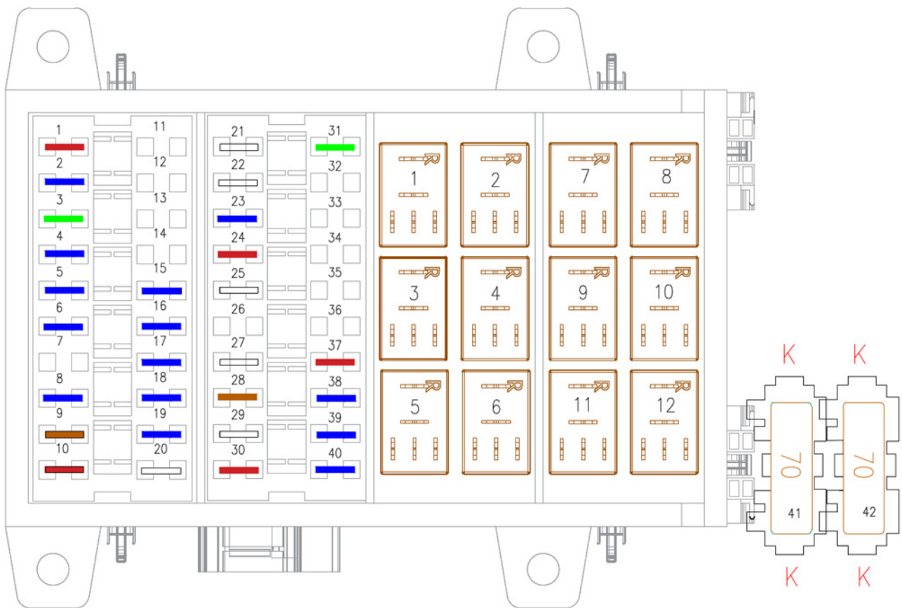
Fig. 5.4.3 Fuse and relays layout in fuse box
