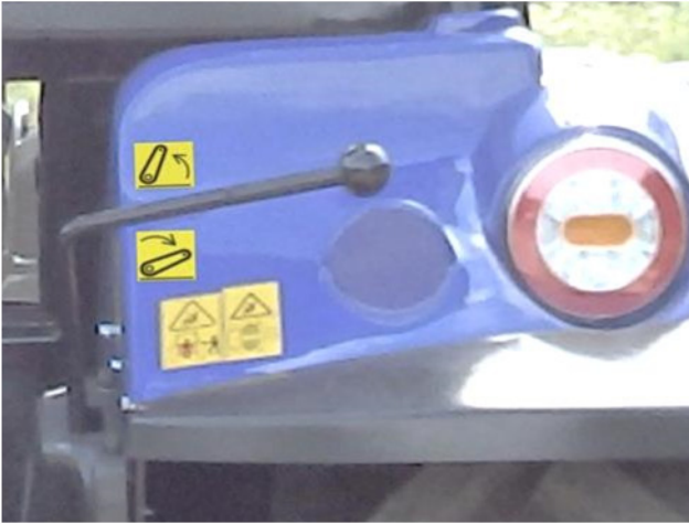
Fig. 4.3.1 Hydraulic lift Hydraulic lift system external control lever
