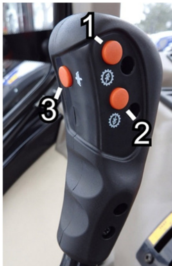
Fig. 3.6. Gear lever with power shift buttons. 1- button for increasing speed / decreasing torque, 2- button for decreasing speed / increasing torque, 3- button for semi-automatic gear change.
