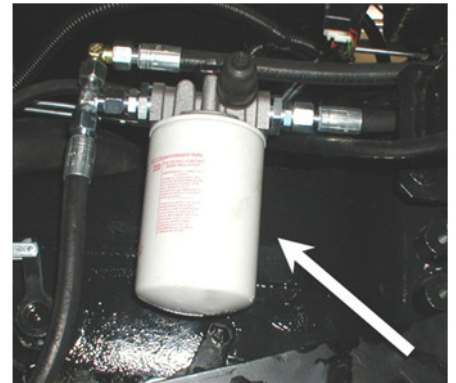
Fig. 5.9.3. Hydraulic oil filter secondary.
