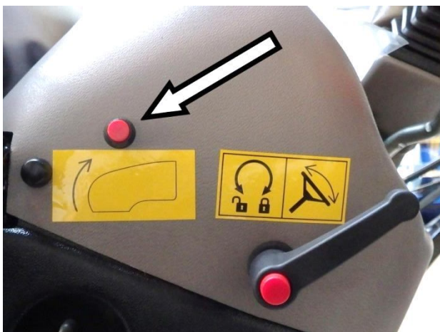
Fig. 4.10. Engine bonnet electromagnetic lock release button.
