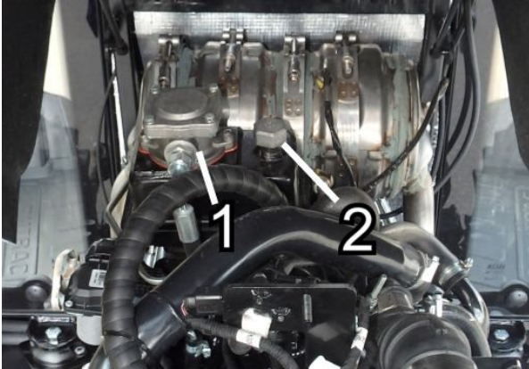
Fig. 5.5.1. Hydrostatic steering oil reservoir: 1 - Oil reservoir housing. 2 - Filler plug with oil level dipstick.
