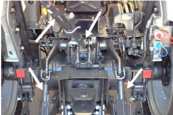
Fig. 5.10. Three-point linkage greasing points
